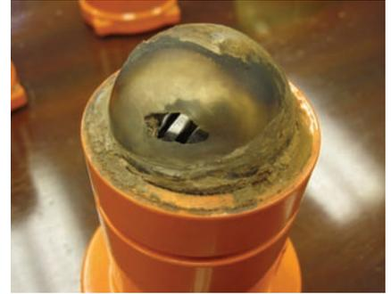
Figure 2. Detectors that protrude into ducts can be rendered ineffective by abrasion from material flow in very short periods of time. These internal components are now exposed to the conveyor's environment. Source: Industrial Fire Prevention LLC.
