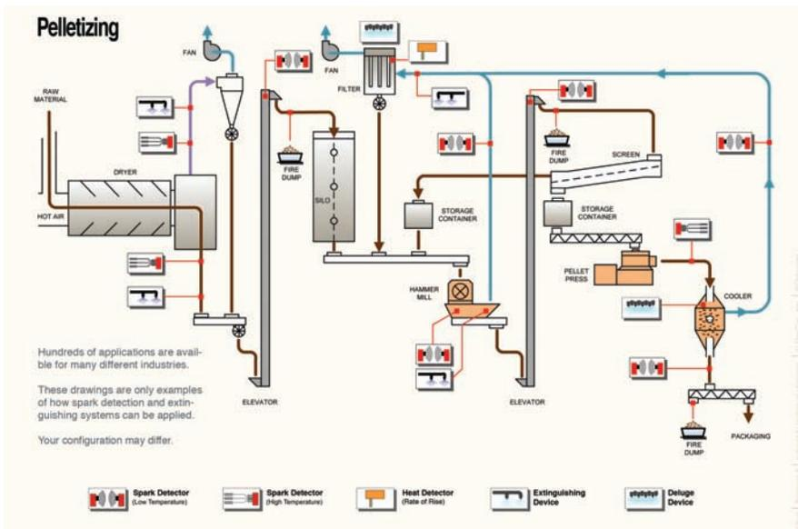
Figure 5. A large plant such as this pelletizing mill may include many IR spark detectors and other types of detectors triggering countermeasures.
