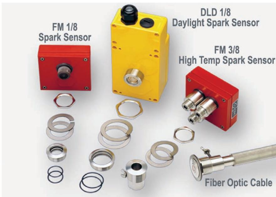
Figure 1. Infrared detectors (FM 1/8 and FM 3/8) by GreCon are capable of detecting sparks in material flows up to 1200°F using fiber optic cables. The blackbody radiation detector (DLD 1/8) is available for standard, high-temperature, and special applications. Detectors shown here include mounting adaptors.
